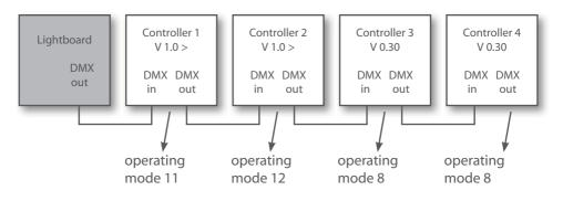
Configuration 2: Dimming function of each output (See also configuration 3)
