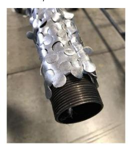
2. With the Circular Base face up, screw in threaded pipe by hand until snug.
