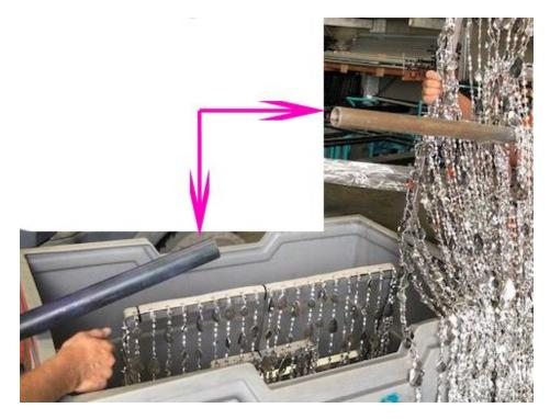
7. Insert the pipe piece of the preassembled 30" square frame inside the dipped down threaded pipe assembly fully until the top of the preassembled square frame is flush with the top of the threaded pipe assembly.
