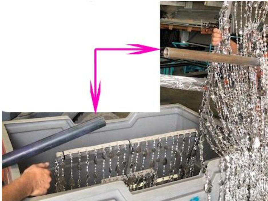
7. Insert the pipe piece of the preassembled 30" square frame inside the dipped down threaded pipe assembly fully until the top of the preassembled square frame is flush with the top of the threaded pipe assembly.
